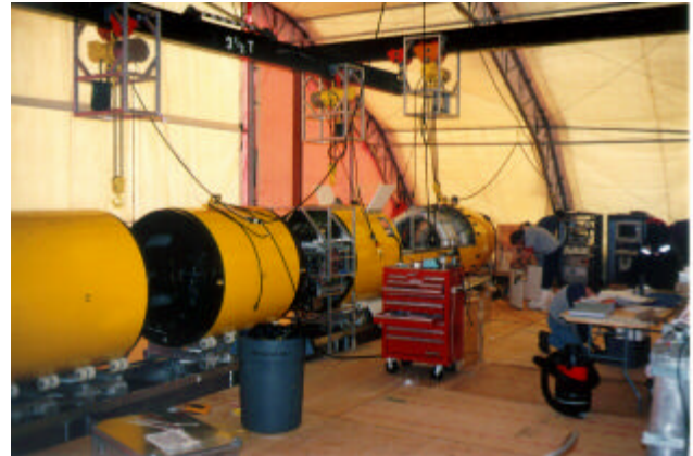
Figure 13. Theseus pulled into segments on its track. Note also the transverse gantry suspended between the two main I-beams.
