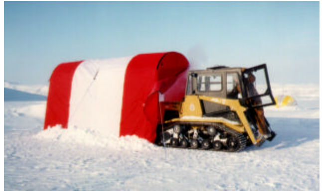
Figure 16. The Posi-Track, kept out of the wind in this thin-walled shelter, would usually start without external heating.
