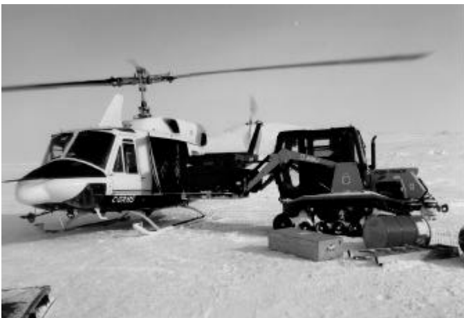
Figure 15. Posi-Track unloading helicopter
