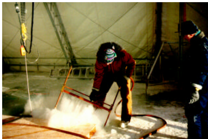
Figure 12. Cutting slots in the ice with hot water.
