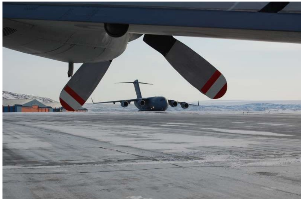
The C17 in the background. The four jet engines, the high tail and the drooping wings are give-aways.
