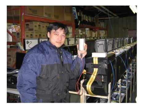
earth shakes, the two of them move relative to one another, and this produces a voltage, which is amplified and recorded. You can see the red cable leading back to the black box. This box contains the recording unit and batteries. Since the recorder works only to minus 20 C, the box is well insulated, and the recorder is surrounded by hot packs to help keep it warm. There is no need to keep the seismometer warm.
