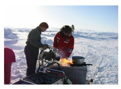
have had a great tea party, but we forgot the tea. One pot-full of water was just sufficient to enlarge the hole enough to pull up the modem (a tube about 5 inches in diameter and about 2 ft long. Low tech to the rescue.
